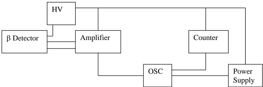
**Figure 7.1:** Component of Beta particle detection system
