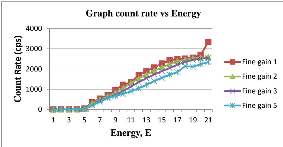
**Figure 5:** The plotted graph of counts/s versus E (energy channel) for various fine gain.
