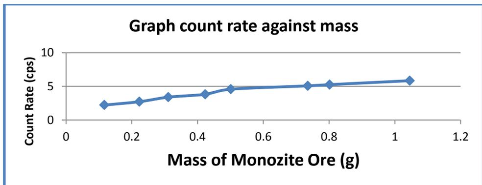
Figure 10 shows that the graph plotted is almost linear, the counts/s is proportionally increasing with weight (g) of Monazite
