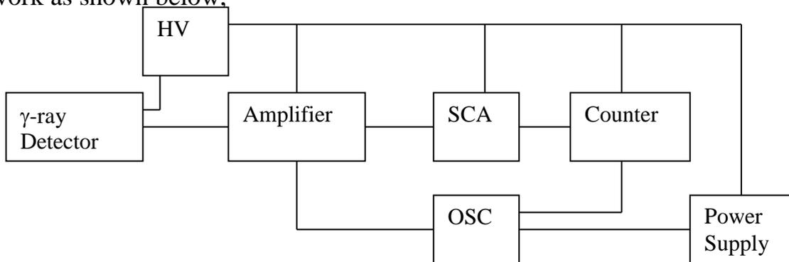
**Figure 4:** Component of gamma ray detection system
