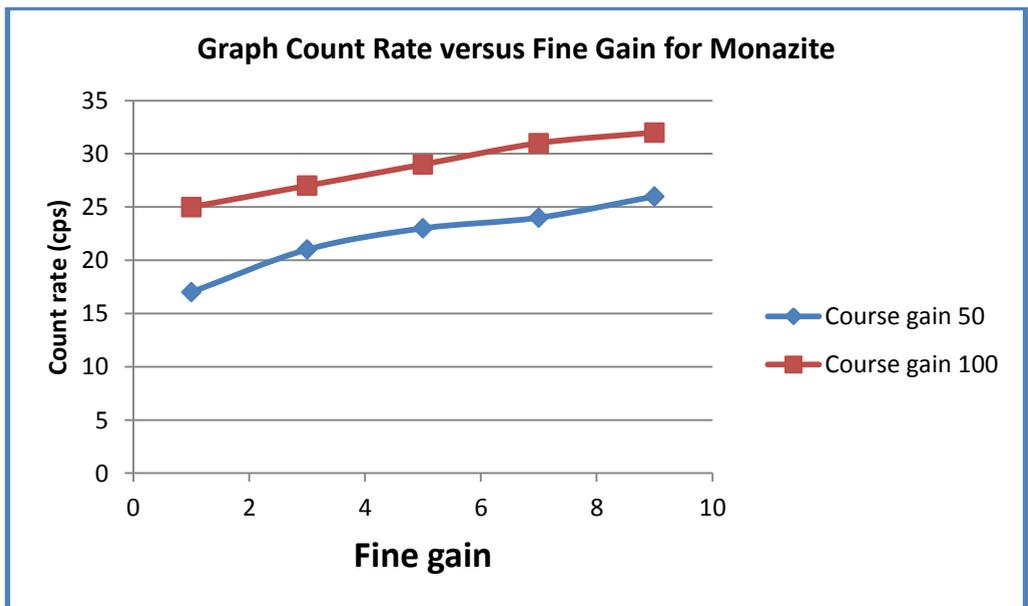
**Figure 8:** Plotted graph of counts versus fine gain for two different course gains
