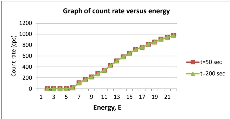
**Figure 6:** The plotted graph of counts/s versus E (energy channel) for a radioactive source Co-60 measured at two different times.
